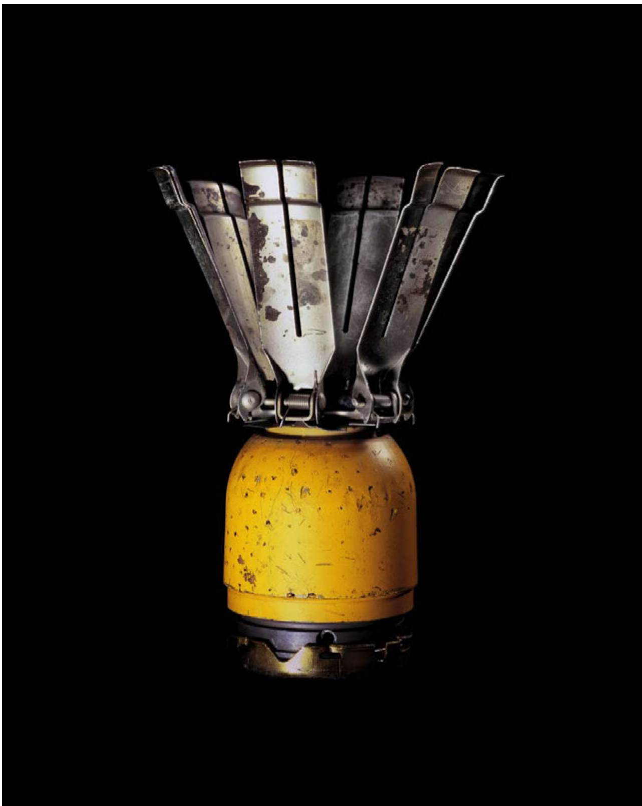
Raphaël Dallaporta, BLU-3 B, États-Unis , tirage Ilfochrome, 30x24 cm, de la série Antipersonnel – Submunition , 2004. On release from a CBU-2C/A bomb this 785g submunition – known as the "Pineapple" – is stabilized and slowed in its descent by six fins. Each CBU-2C/A contains 409 BLU-3/Bs, of which nearly 25 percent do not explode on impact. d : 73 mm wght : 785 g
